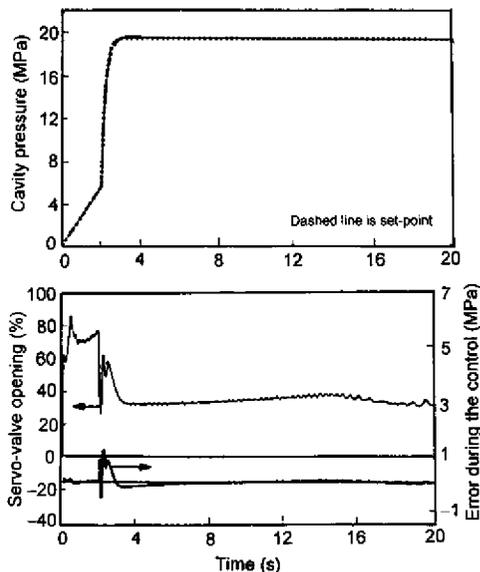
Figure 8. PID Controller tuned with ISE criteria.
