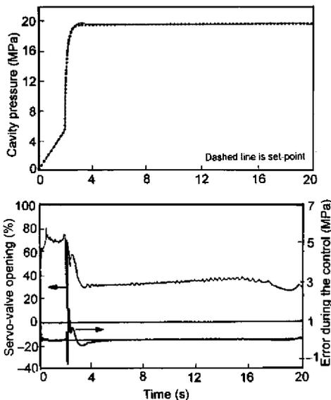
Figure 7. PID Controller tuned with ITAE criteria.
