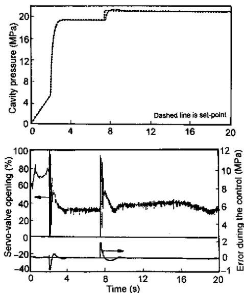
Figure 10. IMC Controller performance to a positive step.
