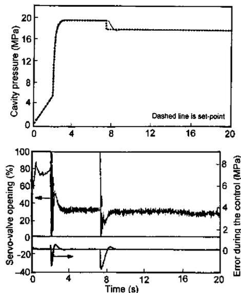
**Figure 11.** IMC Controller performance to a negative step.
