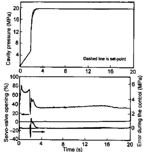
Figure 6. PI Controller tuned with ISE criteria.
