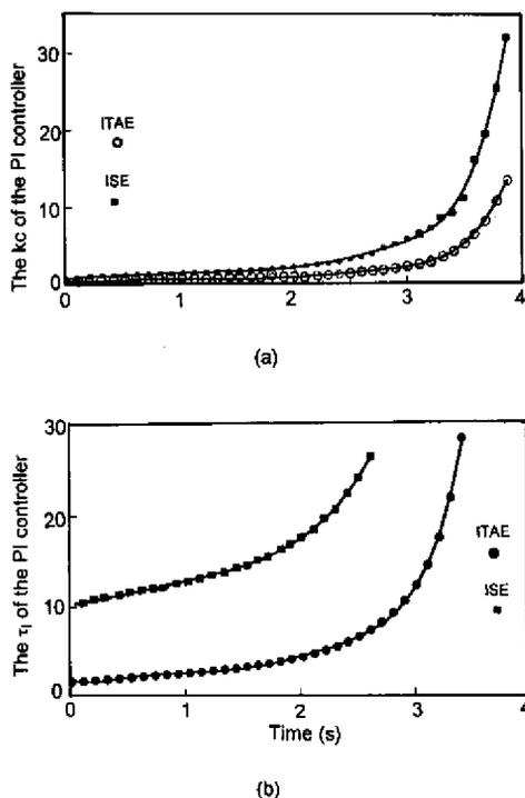
Figure 3. (a) PI Controller gain, (b) PI Controller gain integral time constant.
