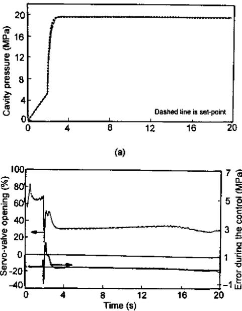
Figure 5. PI Controller tuned with ITAE criteria. (5a) cavity pressure; (5b) servo-valve command and cavity pressure error.
