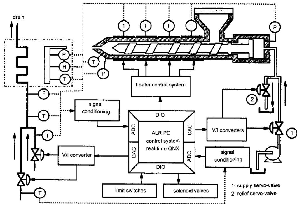
Figure 1. McGill Injection moulding machine.
