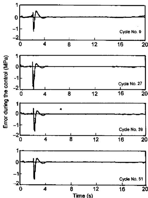
**Figure 12.** Errors of IMC controller in different cycles.
