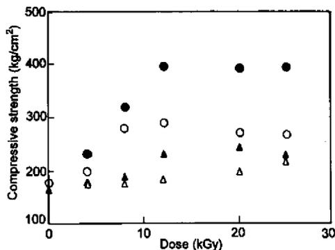
Figure 10. Comparison of compressive strengths of original (solid symbols) and artificially aged (28 days) (open symbols) cedar samples treated with (Δ) AN, (●) AGE/AN. Monomer feed ratio of AGE/AN is 1:1. Compressive strength taken perpendicular to the fibres.
