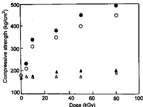
Figure 11. Comparison of compressive strengths of original (solid symbols) and artificially aged (28 days) (open symbols) cedar samples treated with (Δ) MMA, (●) AGE/MMA. Monomer feed ratio of AGE/MMA is 1:1. Compressive strength taken perpendicular to the fibres.
