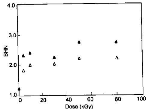
Figure 9. The change of Brinell Hardness Number for cedar samples irradiated in the presence of monomer and monomer mixtures. Monomer feed ratio of AGE/MMA is 1:1. (Δ) MMA, (▲) AGE/MMA.
