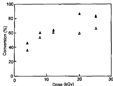
Figure 1. Conversion of monomer and monomer mixtures into homopolymer and copolymer with radiation in cedar. Monomer feed ratio of AGE/AN is 1:1. ( $\Delta$ ) AN, ( $\blacktriangle$ ) AGE/AN.
