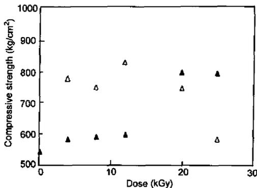
Figure 6. Compressive strength of cedar impregnated with monomer and monomer mixtures depending on the irradiation dose. Monomer feed ratio of AGE/AN is 1:1. Compressive strength taken parallel to the fibres. ( $\Delta$ ) AN, ( $\blacktriangle$ ) AGE/AN.
