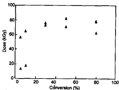
Figure 2. Conversion of monomer and monomer mixtures into homopolymer and copolymer with radiation in cedar. Monomer feed ratio of AGE/MMA is 1:1. ( $\Delta$ ) MMA, ( $\blacktriangle$ ) AGE/MMA.
