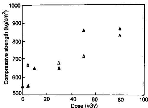
Figure 7. Compressive strength of cedar impregnated with monomer and monomer mixtures depending on the irradiation dose. Monomer feed ratio of AGE/MMA is 1:1. Compressive strength taken parallel to the fibres. (Δ) MMA, (▲) AGE/MMA.
