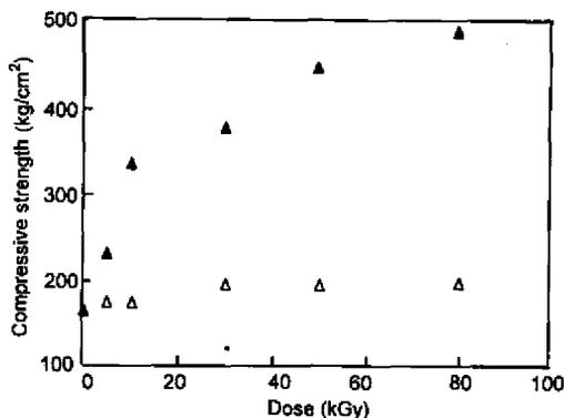
Figure 5. Compressive strength of cedar impregnated with monomer and monomer mixtures depending on the irradiation dose. Monomer feed ratio of AGE/MMA is 1:1. Compressive strength taken perpendicular to the fibres. ( $\Delta$ ) MMA, ( $\blacktriangle$ ) AGE/MMA.
