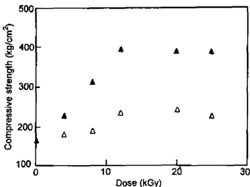
Figure 4. Compressive strength of cedar impregnated with monomer and monomer mixtures depending on the irradiation dose. Monomer feed ratio of AGE/AN is 1:1. Compressive strength taken perpendicular to the fibres. ( $\Delta$ ) AN, ( $\blacktriangle$ ) AGE/AN.
