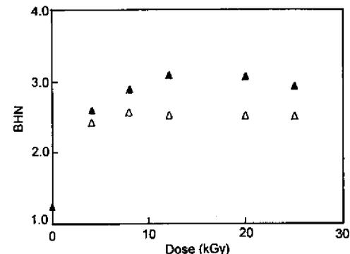
Figure 8. The change of Brinell Hardness Number for cedar samples irradiated in the presence of monomer and monomer mixtures. Monomer feed ratio of AGE/AN is 1:1. (Δ) AN, (▲) AGE/AN.
