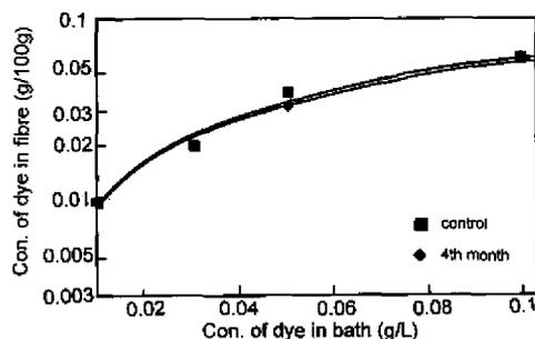
Figure 17. The difference between adsorption isotherms of Chlorantine Fast Green BLL for control and 4 months stored strict middling white cotton bolls.
