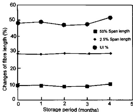
Figure 14. Changes of length of fibres by storage period for middling white cotton fibre.
