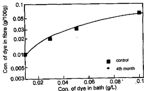
Figure 16. The difference between adsorption isotherms of Chlorantine Fast Green BLL for control and 4 months stored middling white cotton fibres.
