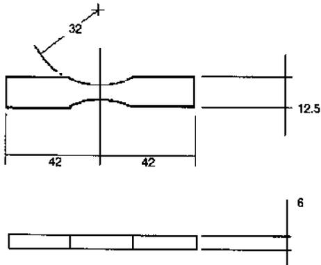
**Figure 2.** Specimen dimensions of the bar used for tensile and flexural fatigue testing in mm.
