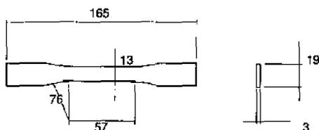
Figure 1. Specimen dimensions of D638 type bar in mm.
