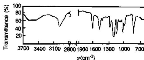
Figure 1. Infrared spectrum of the starting 3D-20 epoxide-diane resin.
