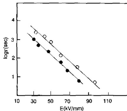
Figure 4. The dependence of the compounds lifetime on the voltage.
