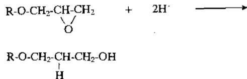
As a result, the complicated aromatic diol is formed: (CH<sub>3</sub>)<sub>2</sub>C[C<sub>6</sub>H<sub>4</sub>O(CH<sub>2</sub>)<sub>n</sub>OH], where n=2, 3, which is used as the stabilizer for ∅D-20 resin-based epoxide compounds.
