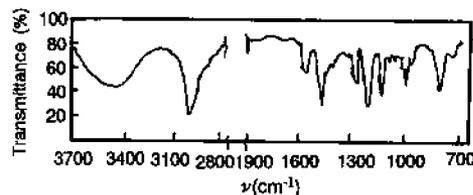
Figure 2. Infrared spectrum of the thermal destruction product (stabilizer).
