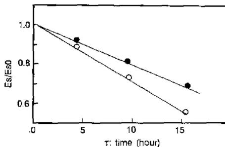
Figure 3. The dependence of the relative electrical strength on the electrical ageing time.
