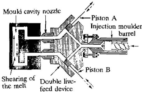
Fig.1. Schematic diagram of one embodiment of a two live-feed device [1,2].
