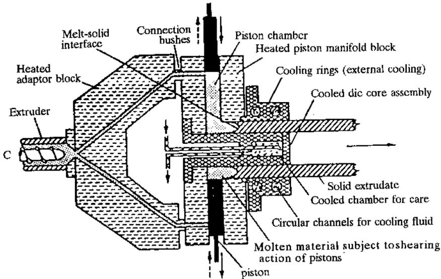
Fig.6(a). Schematic diagram of the centre section through the SCOREX die assembly used for the production of tubes [8]. On this tube die there are four pistons spaced at equal intervals, with two normal to the plane of the diagram, not shown. The appropriate sequencing of the operation of the pistons produces circumferential alignment of fibres and molecules.
