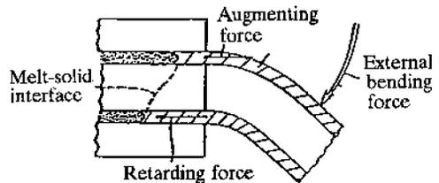
Fig.6(b). Schematic diagram of one arrangement for the production of curvilinear extrusions.
