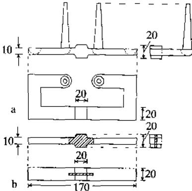
Fig.2(a). The mould geometry used to investigate the effect of change in section thickness [7].
