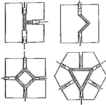
Fig.7. Illustrative example of SCOREX dies that provide for management of orientation in profile extrusion.
