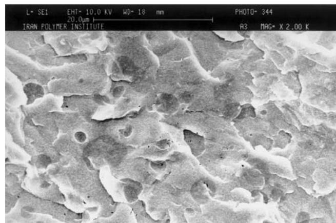
**Figure 7.** SEM Micrograph of the sample containing 5% ATH.
