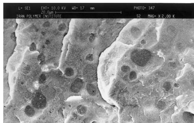
**Figure 8.** SEM Micrograph of the sample containing 4.5% Sb<sub>2</sub>O<sub>3</sub>.
