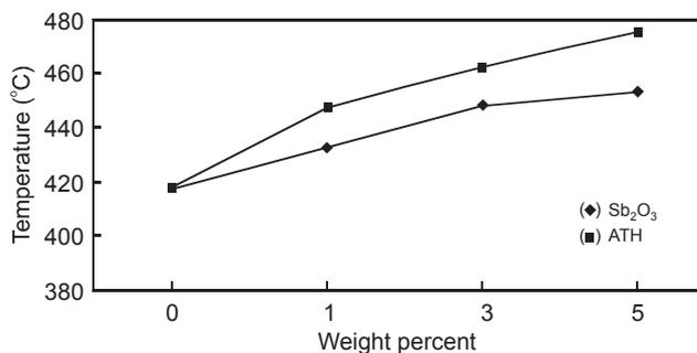
**Figure 6.** Temperatures for 90% weight loss versus the amount of synergist.
