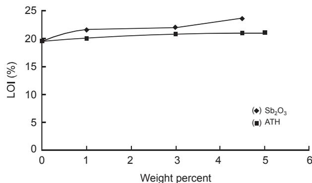
**Figure 1.** Limiting oxygen index amounts for samples containing different weight percent of  $\text{Sb}_2\text{O}_3$  & ATH.
