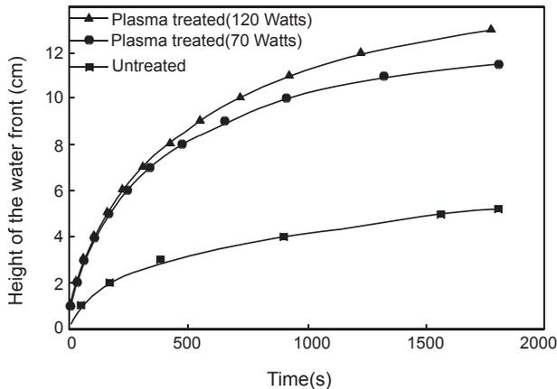
**Figure 4.** The effect of oxygen plasma treatment on the vertical wicking of cotton fabrics.
