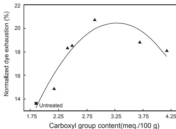
**Figure 3.** The effect of change in cotton carboxyl group contents on direct dye exhaustion of the plasma treated (70 Watts power, 30 mL/min oxygen gas flow rate, 60 min) cotton fibres (dyed in distilled water, LR  $\approx$  40:1, at 60°C, and for 60 min).
