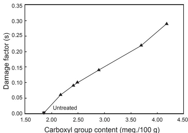
**Figure 2.** The relation between the carboxyl group contents of the plasma treated cotton fibres and the damage caused by the plasma treatment (70 Watts power, 30 mL/min oxygen gas flow rate, 60 min).
