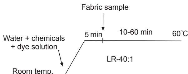
**Figure 1.** Schematic chart of dyeing processes.
