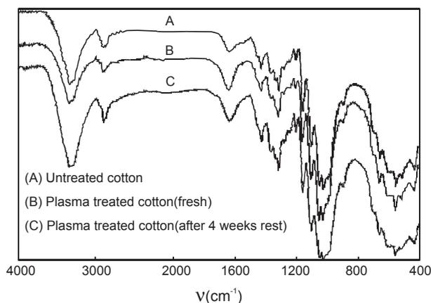
**Figure 6.** FTIR Spectra recorded from the untreated, oxygen plasma treated (70 Watts power, 30 mL/min gas flow rate, 60 min), and aged oxygen plasma treated cotton samples.
