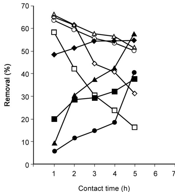
**Figure 2.** Plots of percentage removal of suspended solid of sewage vs. contact time with polymer dose. (□) 0.4 mg/L; (○) 0.8 mg/L; (△) 1.2 mg/L; (◇) 1.6 mg/L.
