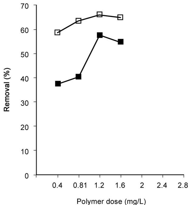
**Figure 1.** Plots of percentage removal of suspended solid sewage (□) and Tannery (■) vs. polymer dose at temperature = 32°C.
