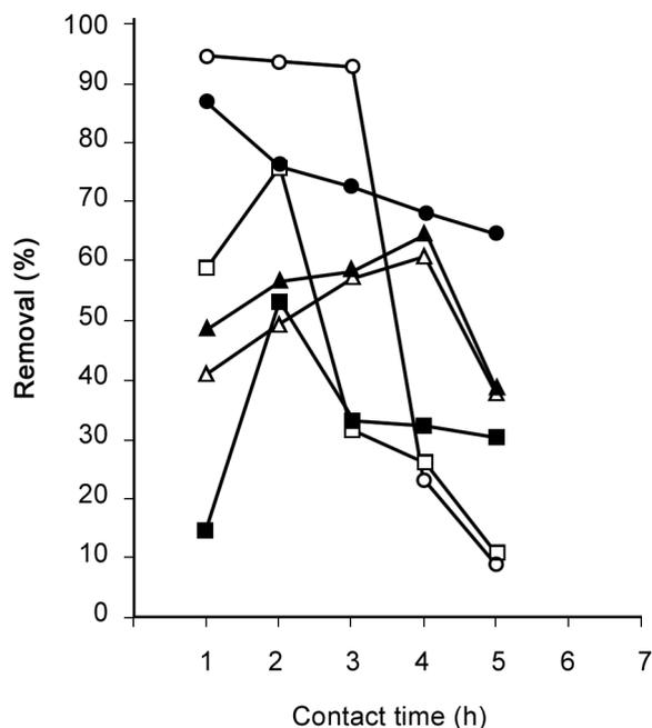
**Figure 3.** Plots of percentage removal of suspended solid of sewage vs. contact time. Polymer dose = 1.2 mg/L; pH (□)4.0; (○) 7.0; (△)9.2.
