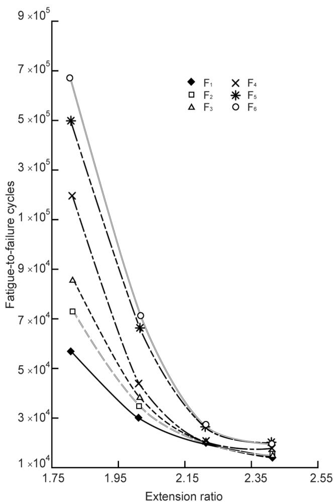
Figure 1. Plot of fatigue-to-failure cycles against VTEOS content.
