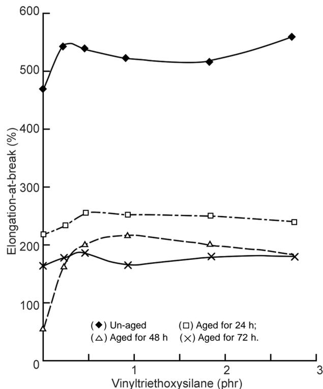
Figure 5. Plot of elongation-at-break against VTEOS concentration with different aging time.
