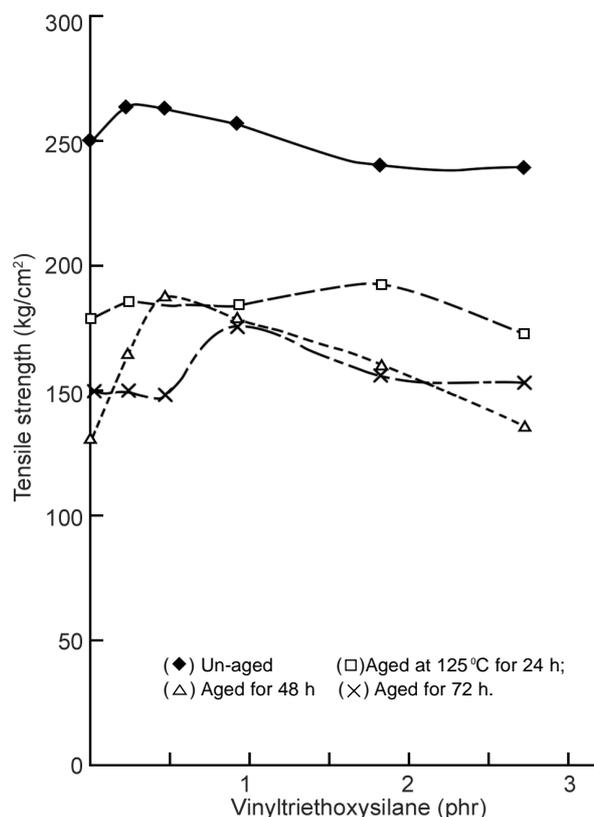
Figure 4. Plot of tensile strength against VTEOS concentration.
