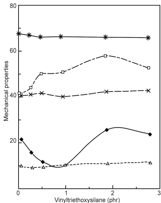
(◆) Compression set(%); (□) Tear strength(kg/cm); (△) Abrasion resistance (cc/1000); (×) Resilience (% rebound); (\*) Hardness (shore A).
