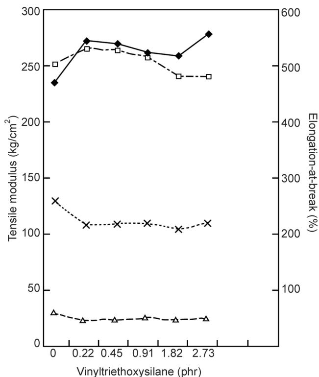
(□) Tensile strength; (△) Modulus at 100% elongation; (×) Modulus at 300% elongation; (◆) Elongation-at-break.
