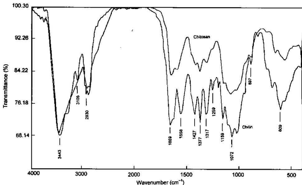
Figure 1. FTIR Spectra of chitin and chitosan (PGC).
