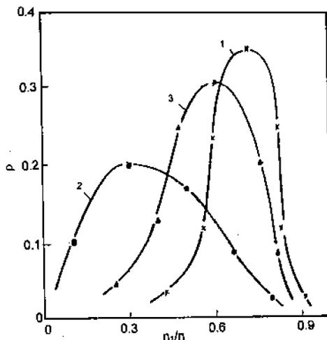
Figure 3. Differential curves of distribution density of Na-CMC on degree of substitution: (1) Na-CMC prepared from viscose cellulose; (2) from wastes of cotton-gin plants; (3) from wastes of cotton-gin plants with addition of mass-diffusion microaccelerator.
