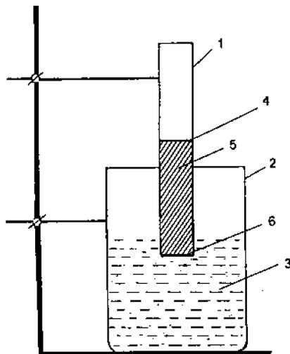
Figure 2. Laboratory apparatus for determination of coefficients of mass-diffusion, of cellulose raw materials in the systems -solid substance -liquid: (1) tube; (2) glass; (3) alkaline solution; (4) fixer of alkali; (5) cellulose containing material; (6) surface of phase contacts.
