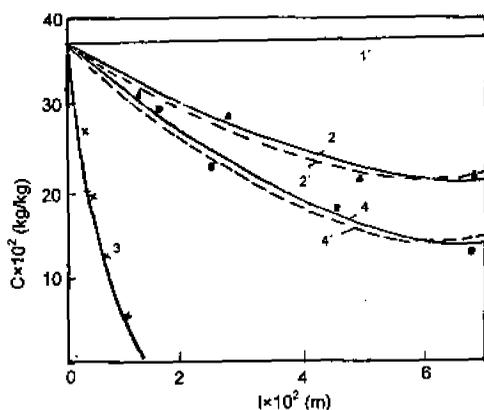
Figure 4. Curves of mass-diffusion of cellulose raw materials: (1) materials at  $D=\infty$ ; (2&2') experimental and estimated curves of viscose cellulose; (3) wastes of cotton-gin plants; (4&4') experimental and estimated curves of wastes of cotton-gin plants after addition of microaccelerator.
