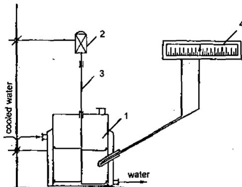
Figure 1. Laboratory apparatus for synthesis of Na-CMC: (1) reactor; (2) electromotor; (3) mixer; (4) device for temperature measurement.
