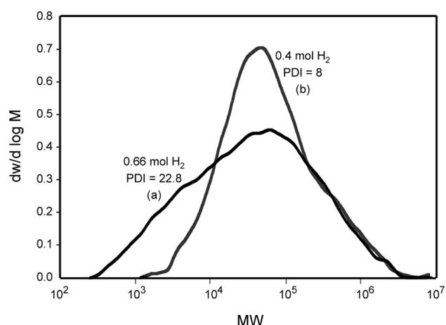
**Figure 1.** Effect of hydrogen amount added in the first step on MW and MWD: (a) 0.66 mol H<sub>2</sub> (sample No. 6), and (b) 0.4 mol H<sub>2</sub> (sample No. 2).
