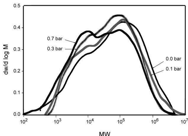
**Figure 6.** Effect of comonomer amount added in the second step on MW and MWD in the presence of 0.66 mol H<sub>2</sub>.
