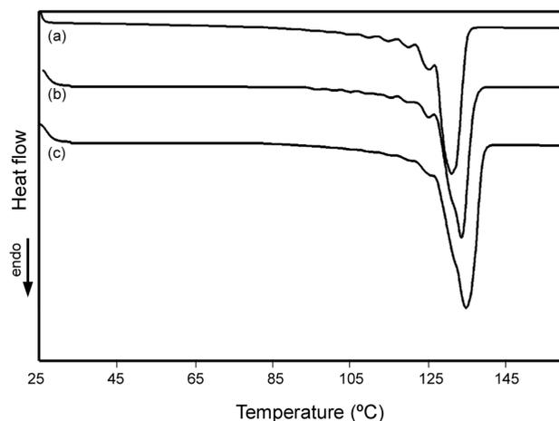
**Figure 7.** DSC-SSA Endotherms of specimens synthesized under different comonomer partial pressures of 0.7, 0.3, 0.1 bar added in the second step for: (a) C1H2-60-10 (No. 8), (b) C2H2-60-10 (No. 9) and (c) C3H2-60-10 (No. 10), respectively.
