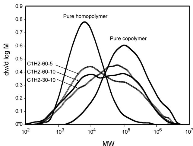
**Figure 4.** Effect of polymerization time of both steps on MW and MWD in the presence of 0.66 mol H<sub>2</sub>.
