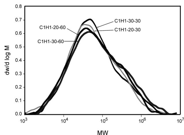
**Figure 3.** Effect of polymerization time of both steps on MW and MWD in the presence of 0.4 mol H<sub>2</sub>.
