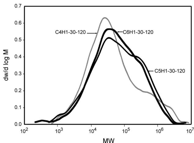
**Figure 5.** Effect of comonomer amount added in the second step on MW and MWD in the presence of 0.4 mol H<sub>2</sub>.
