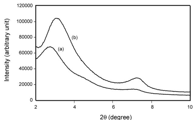
**Figure 1.** XRD Patterns of pristine C-15A: (a) before and (b) after sonication in toluene.
