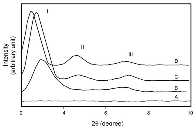
**Figure 4.** Diffraction patterns of nanocomposites containing OPPW. Sample A (no clay), sample B (no wax), sample C (wax:clay is 0.5:1) and sample D (wax:clay is 1:1).
