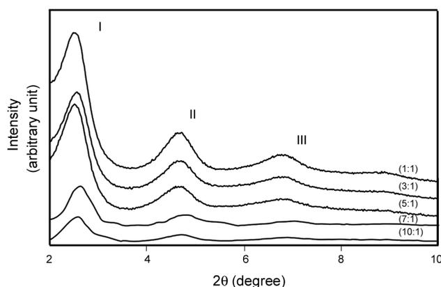
**Figure 3.** Diffraction patterns of the mixtures with different ratios of OPPW-2:C-15A.
