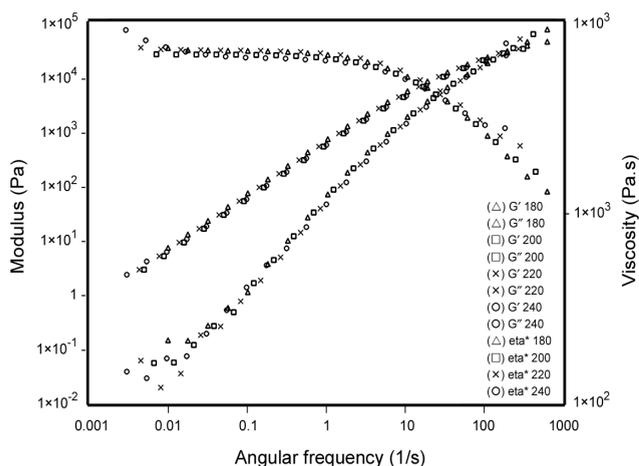
**Figure 5.** The frequency dependence of storage modulus ( $G'$ ), loss modulus ( $G''$ ) and complex viscosity ( $\eta^*$ ) for sample A (no clay).
