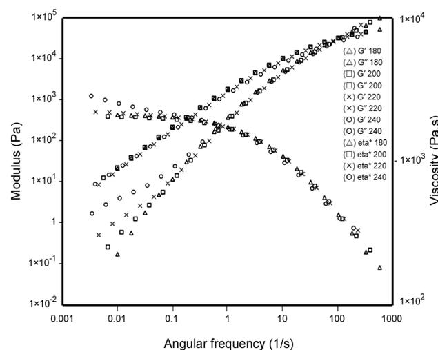
**Figure 7.** The frequency dependence of storage modulus ( $G'$ ), loss modulus ( $G''$ ) and complex viscosity ( $\eta^*$ ) for sample C (wax:clay is 0.5:1).
