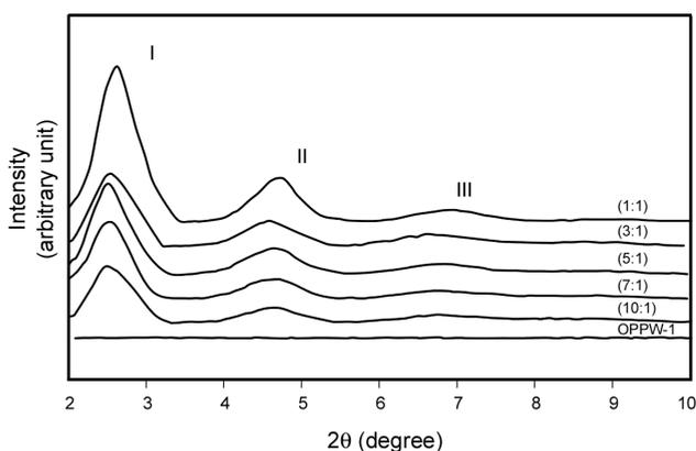
**Figure 2.** Diffraction patterns of neat OPPW-1 and the mixtures with different ratios of OPPW-1:C-15A.
