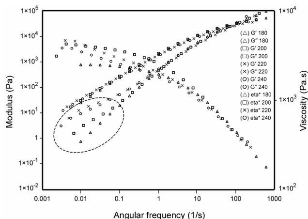
**Figure 8.** The frequency dependence of storage modulus ( $G'$ ), loss modulus ( $G''$ ) and complex viscosity ( $\eta^*$ ) for sample D (wax:clay is 1:1).
