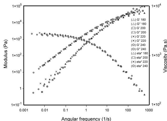
**Figure 6.** The frequency dependence of storage modulus ( $G'$ ), loss modulus ( $G''$ ) and complex viscosity ( $\eta^*$ ) for sample B (no wax).
