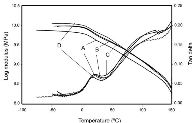
**Figure 10.** The moduli and loss factor curves for samples: A (no clay), B (no wax), C (wax:clay 0.5:1) and D (wax:clay 1:1).
