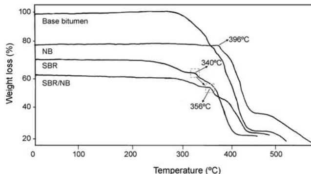
**Figure 4.** TGA weight loss curves of SBR modified bitumen samples before and after the addition of NB.
