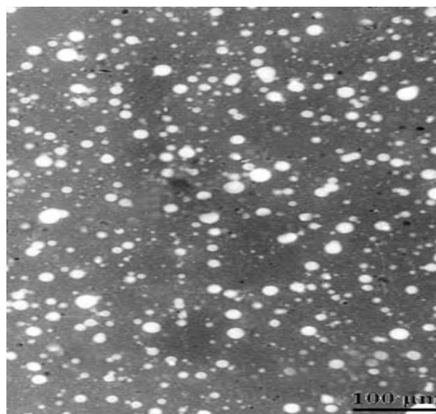
**Figure 10.** Morphology of SBR3%/NB2% modified bitumen by optical microscope.
