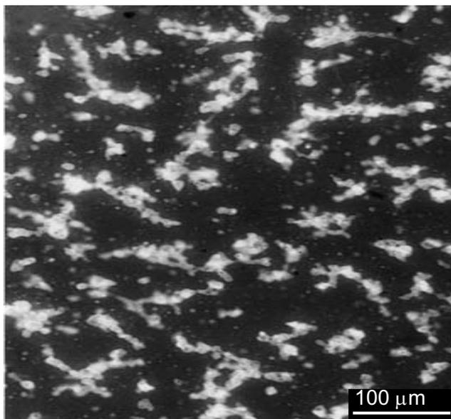
**Figure 11.** Morphology of SBR3%/NB3% modified bitumen by optical microscope.
