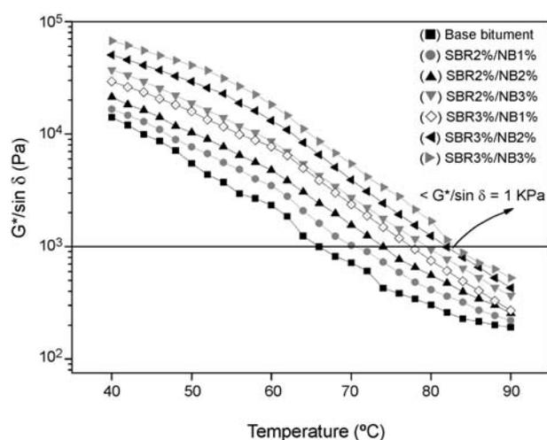
**Figure 3.** Curves of  $G^*/\sin \delta$  vs. temperature for SBR/NB modified bitumen samples.
