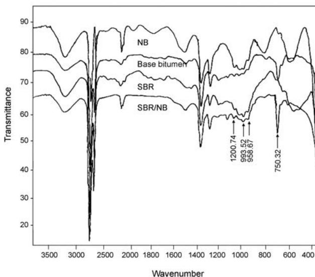
**Figure 7.** FTIR analysis of SBR and SBR/NB modified bitumen samples.
