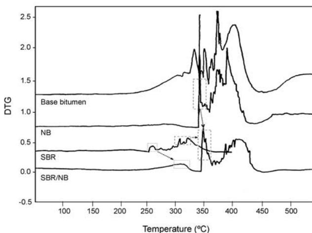
**Figure 5.** DTGA curves of SBR modified bitumen samples before and after the addition of NB.
