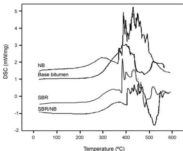
**Figure 6.** DSC tests of SBR and SBR/NB modified bitumen samples.
