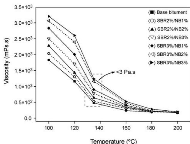
**Figure 2.** Viscosity of bitumen mixings with SBR/NB vs. temperature.
