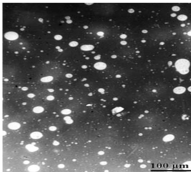
**Figure 9.** Morphology of SBR2%/NB2% modified bitumen by optical microscope.
