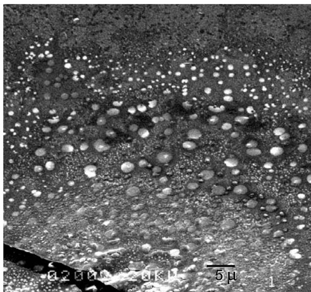
**Figure 13.** Morphology of SBR3%/NB2% modified bitumen by SEM.
