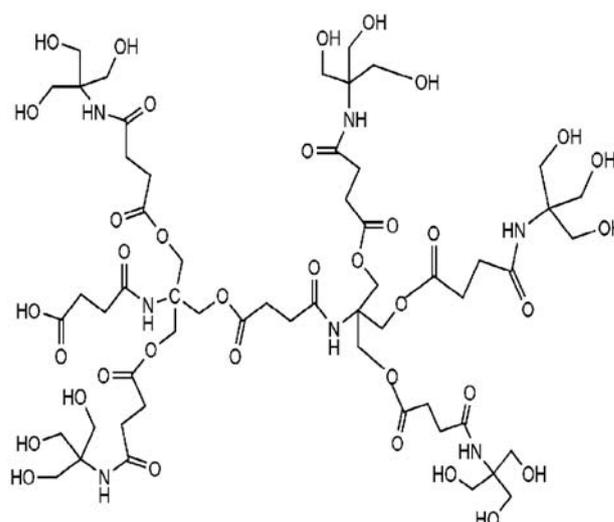
**Figure 1.** Schematic structures of AB<sub>3</sub> hyper-branched poly(amide-ester) (HBP).
