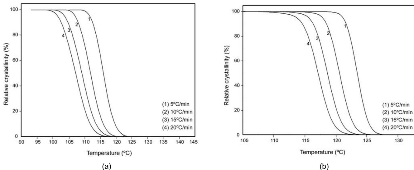
**Figure 3.** Development of relative crystallinity with temperature for non-isothermal crystallization of: (a) iPP and (b) HBP/PP blend ( $\bar{M}_{nHBP} = 7800$  g/mol).
