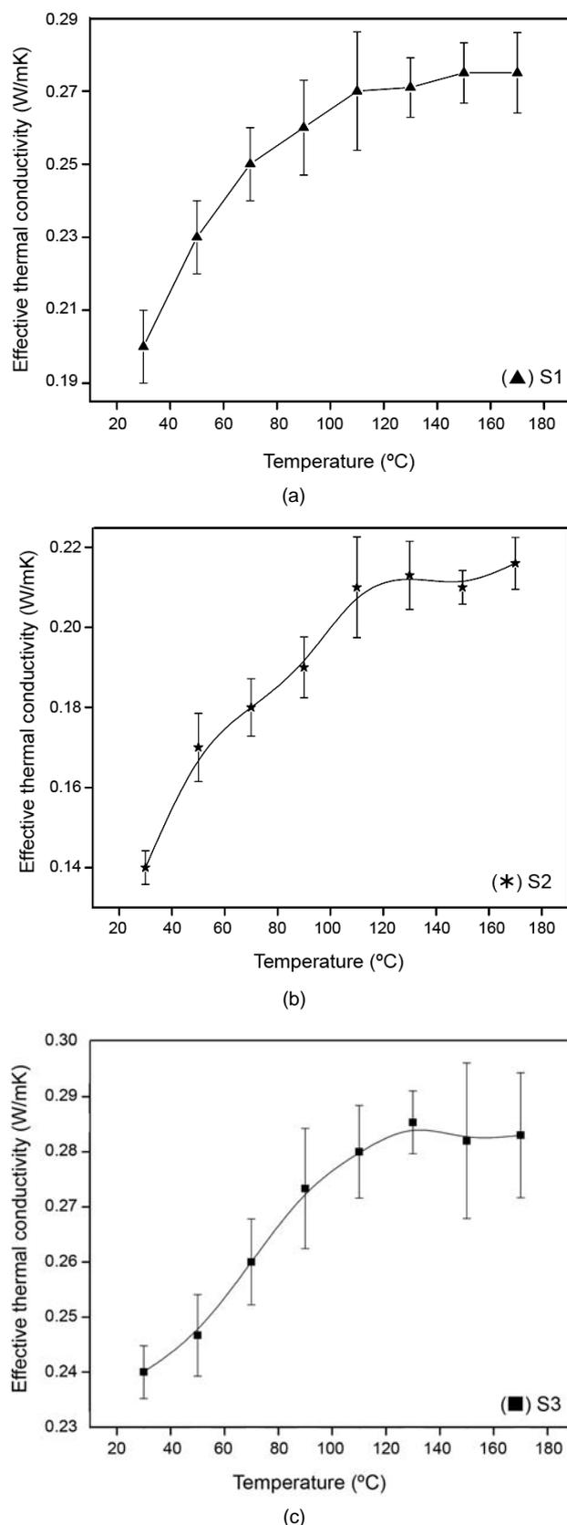
**Figure 7.** Effective thermal conductivities of S1 (a), S2 (b) and S3 (c).
