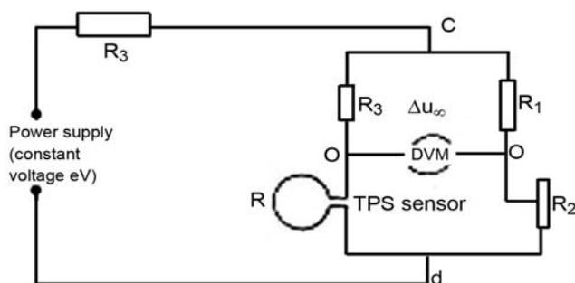
**Figure 5.** Bridge circuit.
