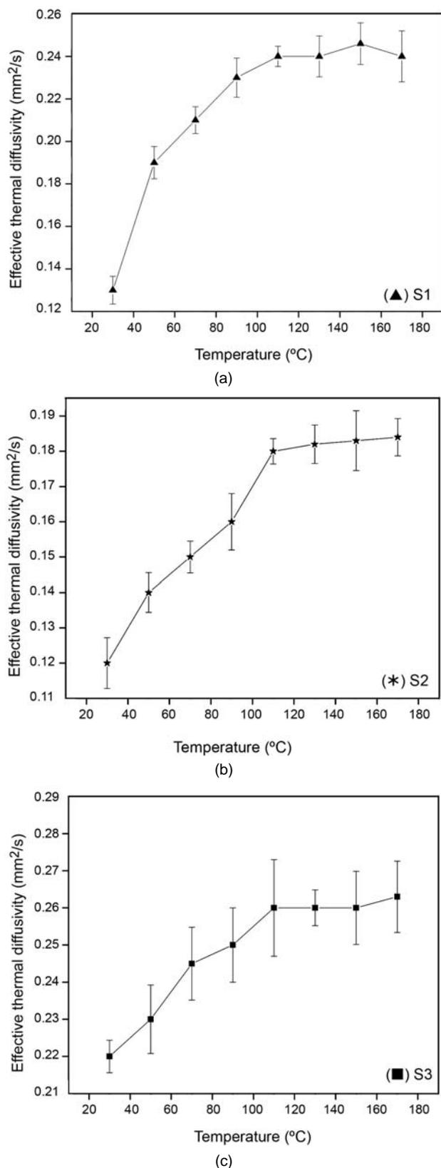
**Figure 8.** Effective thermal diffusivities of S1 (a), S2 (b) and S3 (c).
