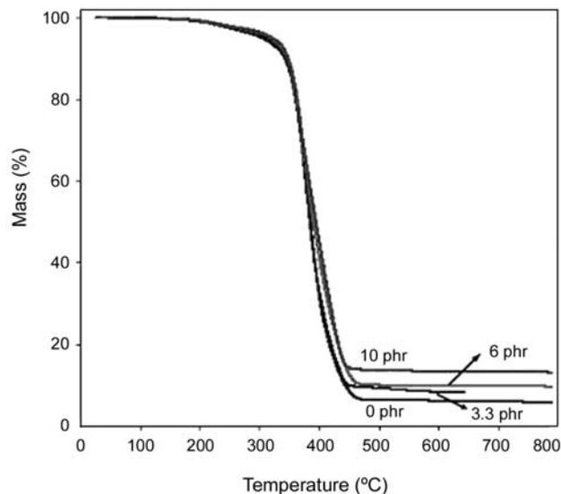
**Figure 7.** TGA Curves of pure NR and NR/Na-MMT nanocomposites.
