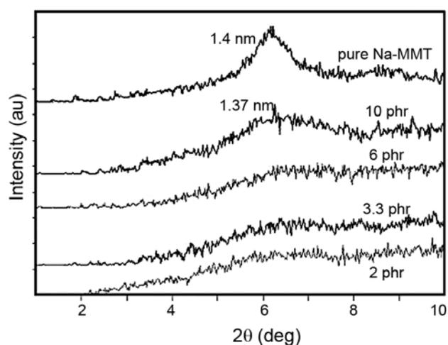
**Figure 1.** XRD patterns for the pure Na-MMT and NR/Na-MMT nanocomposites.
