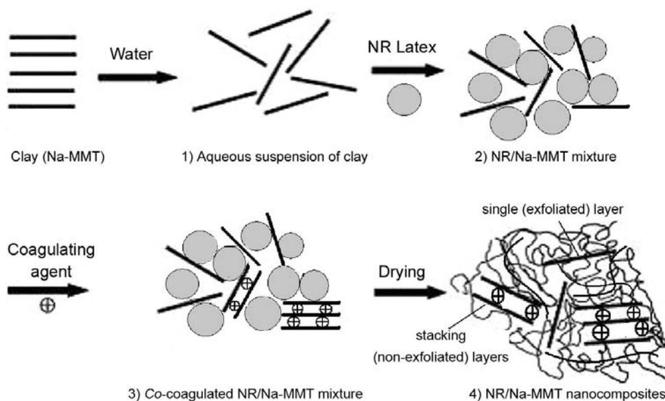
**Figure 4.** Schematic illustration of the mixing and co-coagulating processes [22].
