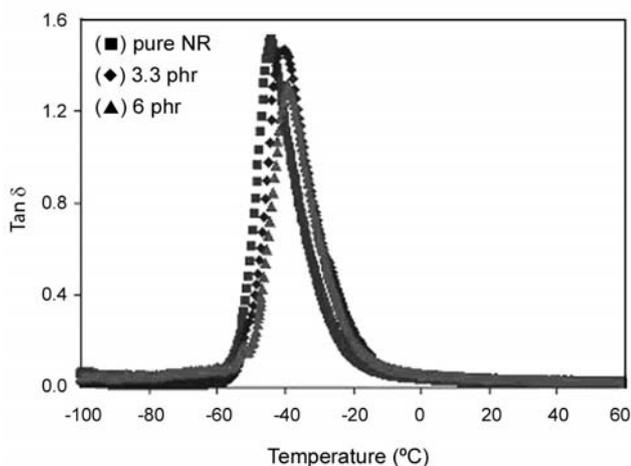
**Figure 6.**  $\tan \delta$  versus temperature for pure NR and NR/ Na-MMT nanocomposites.
