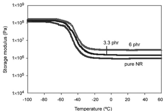
**Figure 5.** The storage modulus versus temperature for pure Na-MMT and NR/ Na-MMT nanocomposites.
