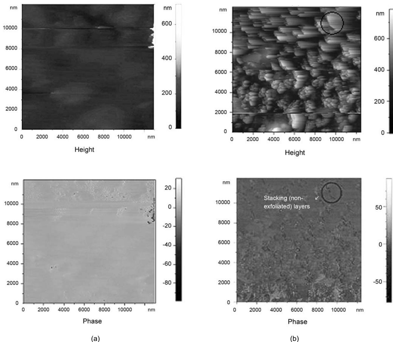
**Figure 2.** AFM Phase images of NR/Na-MMT nanocomposites prepared by co-coagulating the mixture of NR latex and Na-MMT aqueous suspension: (a): 3.3 phr Na-MMT, (b): 10 phr Na-MMT.
