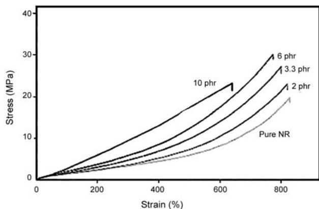
**Figure 8.** Stress-strain curves for pure NR and NR/Na-MMT nanocomposites.
