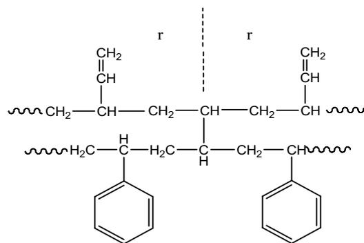
**Scheme VII.** Proposed mechanism of grafting polystyrene on 1,2-polybutadiene
