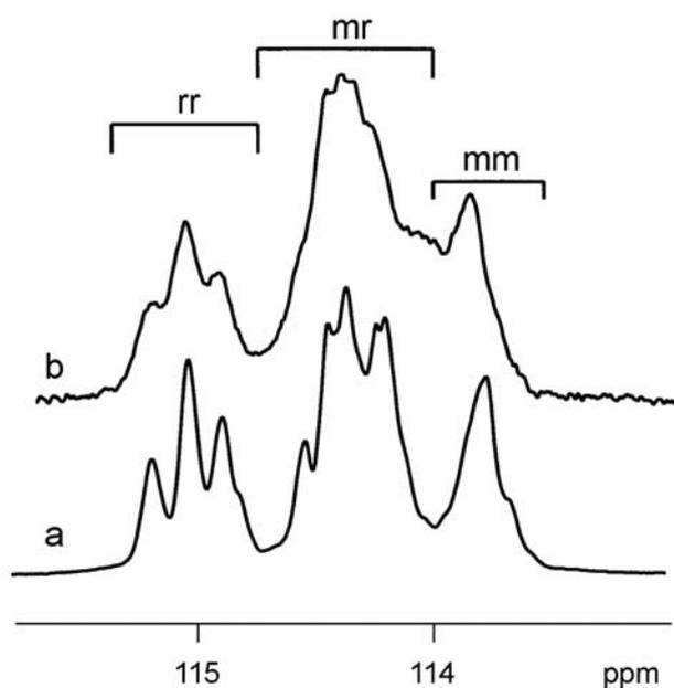
**Figure 11.**  $^{13}\text{C}$  NMR spectrum of olefinic methylene carbon, 1,2-PBD (a) and PS-*g*-1,2-PBD (b) in  $\text{CDCl}_3$  at room temperature.
