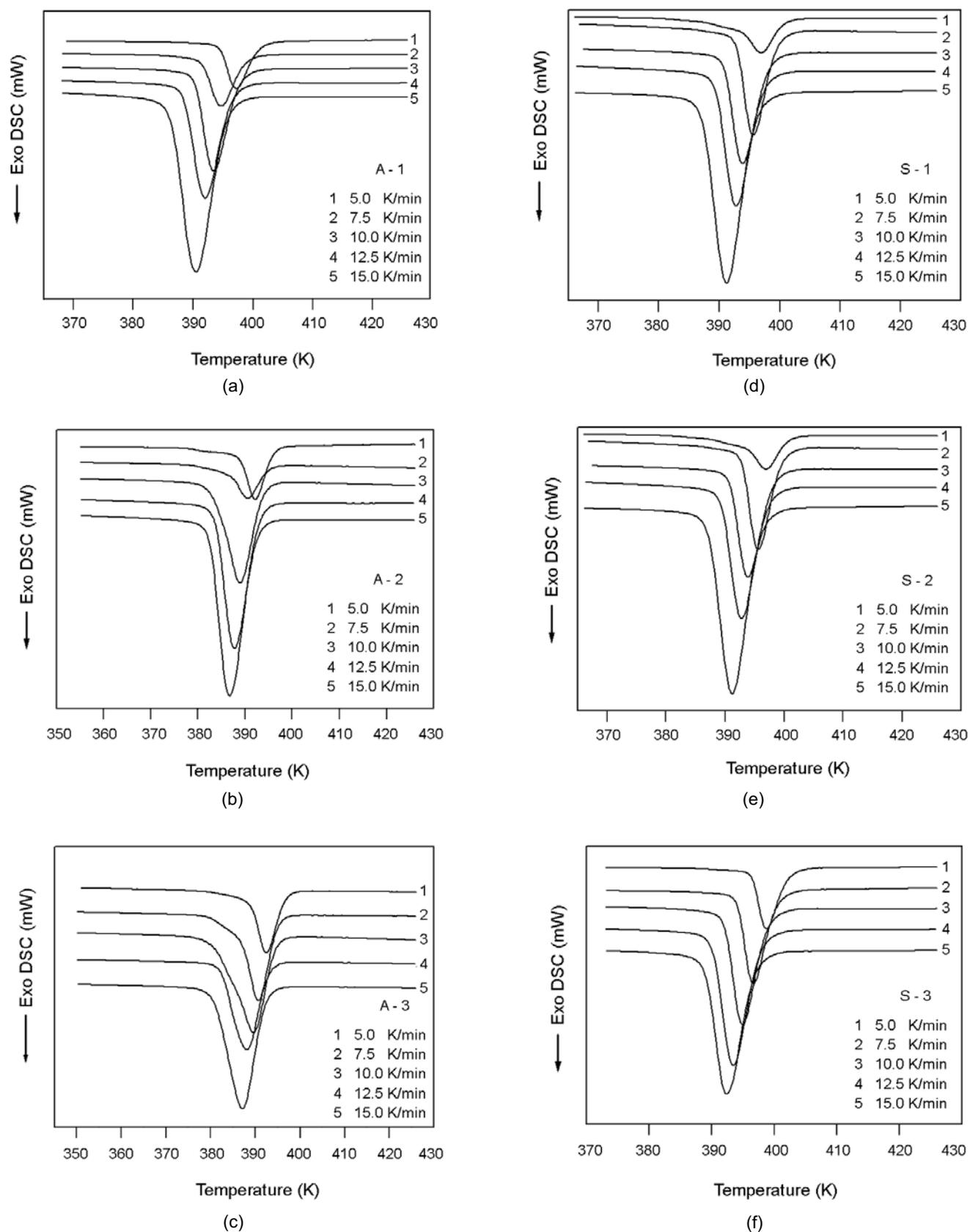
**Figure 1.** DSC Thermograms of: (a) A-1, (b) A-2, (c) A-3, (d) S-1, (e) S-2, and (f) S-3 composites during non-isothermal crystallization at different cooling rates.
