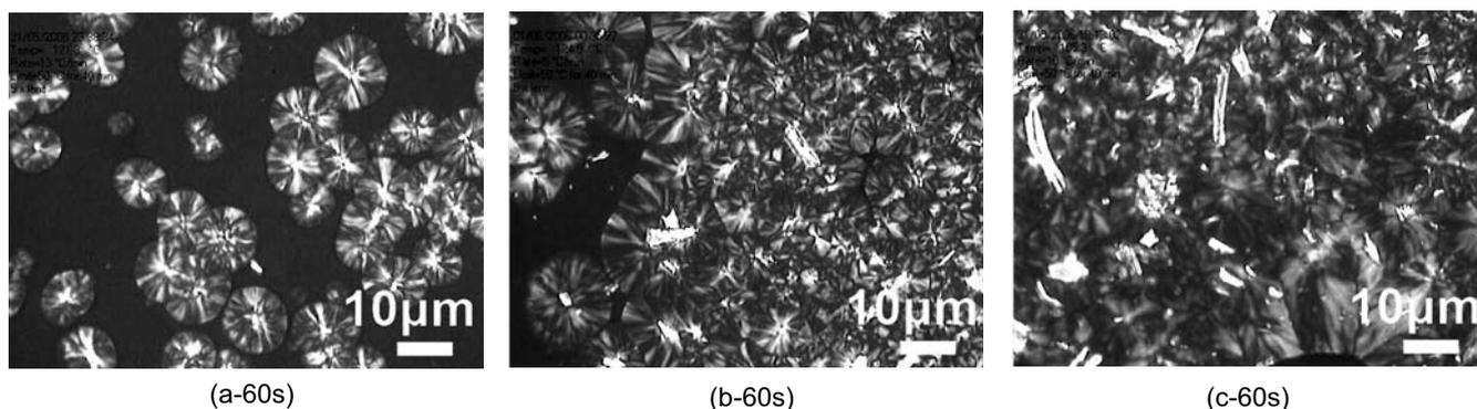
**Figure 6.** Polarized optical micrographs showing the morphology of crystals of: (a) PP, (b) PP/MCC1, and (c) PP/MCC2 composites at various time (magnification  $\times 500$ , crystallizing temperature  $130^{\circ}\text{C}$ ).
