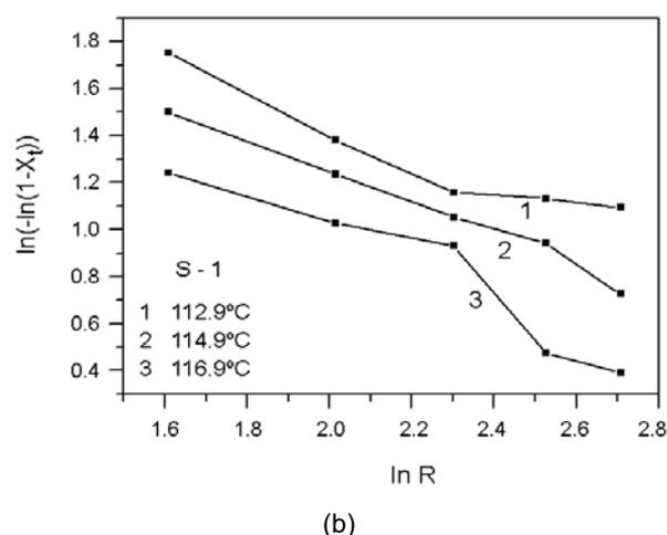
**Figure 4.** Ozawa plots of  $\ln(-\ln(1-X_t))$  vs.  $\ln R$  for crystallization of: (a) A-1 and (b) S-1 composites at different temperature.
