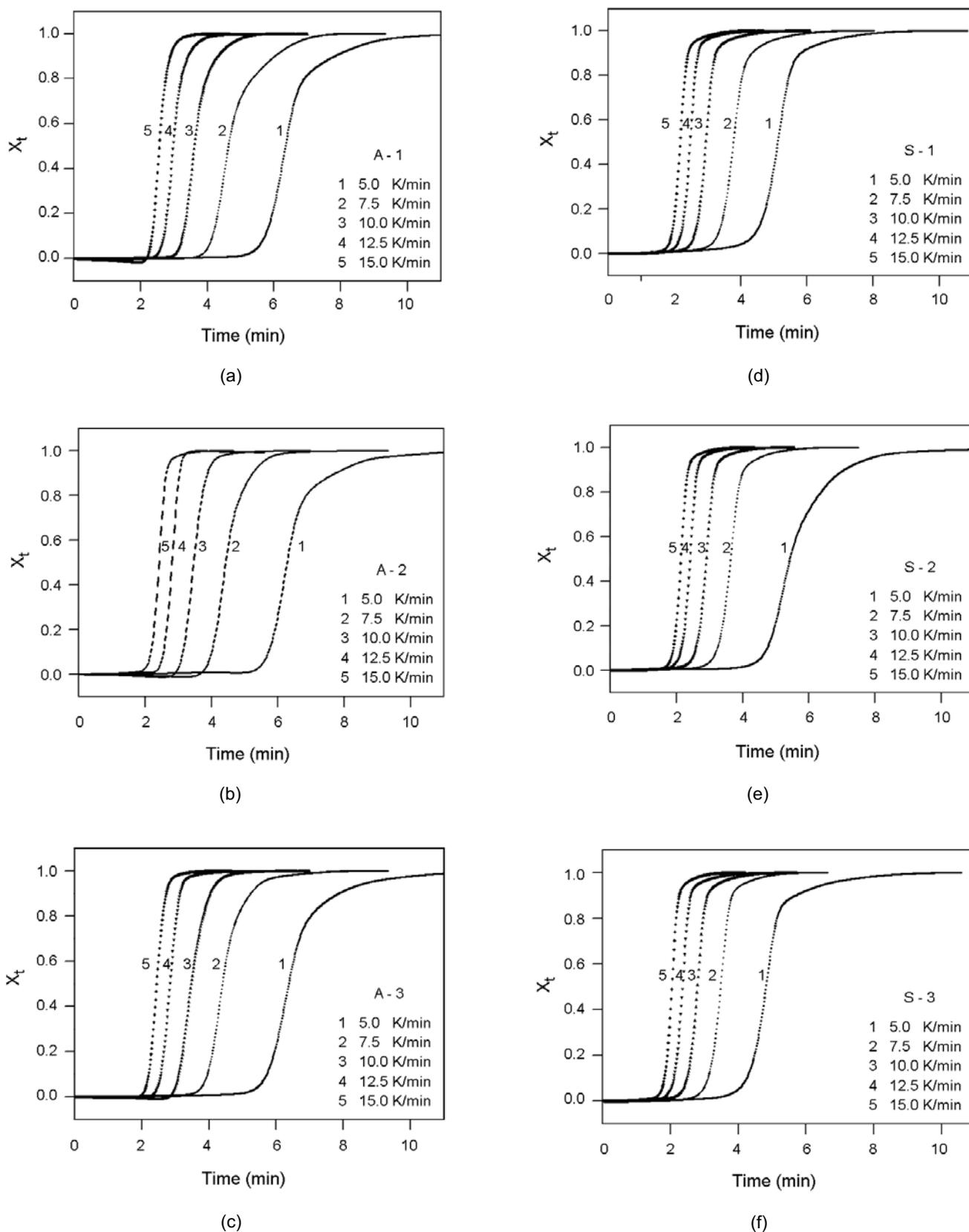
**Figure 2.** Relative crystallinity degree versus time for non-isothermal crystallization of: (a) A-1, (b) A-2, (c) A-3, (d) S-1, (e) S-2, and (f) S-3 composites at various cooling rates.
