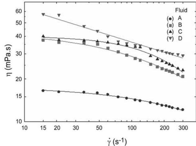
**Figure 2.** Dynamic viscosity data of PAA solutions. Solid lines are the predictions of the modified-upper-convected Maxwell model.
