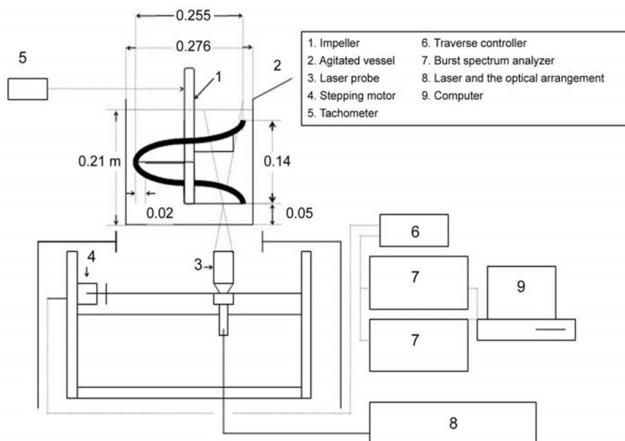
**Figure 1.** Setup of LDA and agitated vessel for mixing of viscoelastic liquids (all dimensions are in meter).
