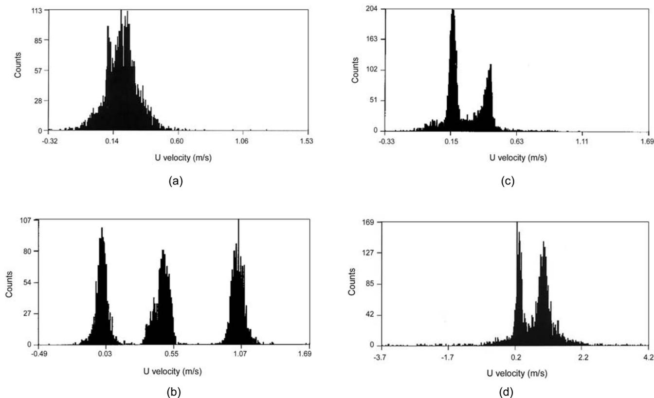
**Figure 3.** Tangential velocity histograms of: (a) fluid A, (b) fluid C, (c) fluid B, (d) fluid D ((Table 1) with helical ribbon impeller).
