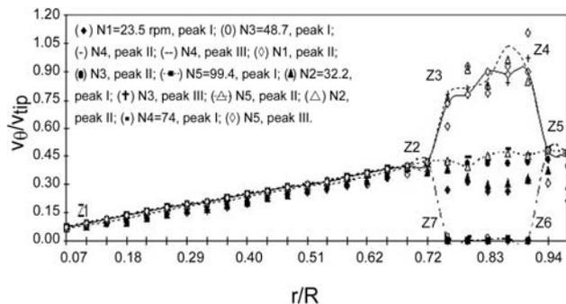
**Figure 4.** Three zone velocity profiles of helical ribbon impeller for 900 ppm PAA solution at different impeller speeds (the peaks I, II and III are the same as that of Figure 3).
