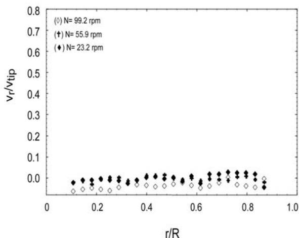
**Figure 7.** Dimensionless radial velocities of helical ribbon impeller versus radial for 1350 ppm PAA solution and different impellers.
