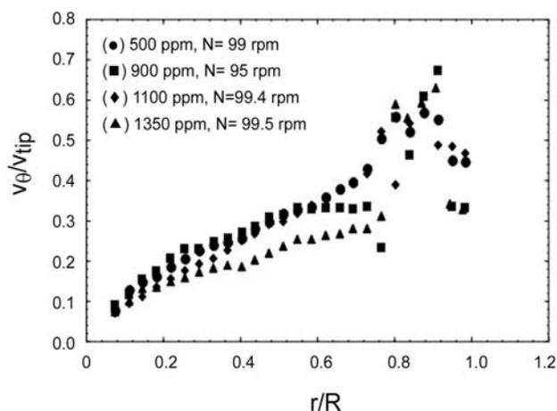
**Figure 6.** Dimensionless tangential velocities for different concentrations of PAA solutions.
