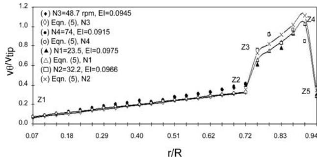
**Figure 5.** Predicted values of eqn (5) for tangential velocity of helical ribbon impeller in mixing of PAA solutions.
