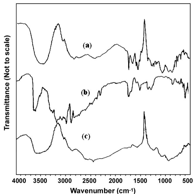
**Figure 1.** FTIR Spectra of: (a) model drug riboflavin, (b) drug-loaded, and (c) blank samples.
