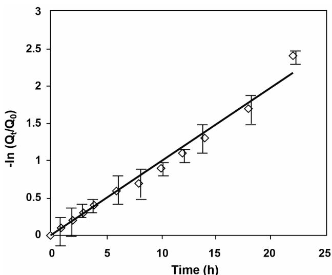
**Figure 5.** First-order kinetic plot of the release of B2 from sample HG (0.58) in SGF of pH 1.2 at 37°C.
