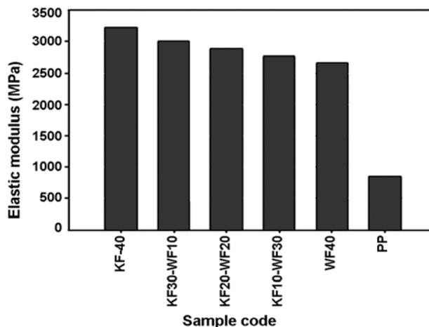
**Figure 1.** Tensile moduli of various composite formulations.
