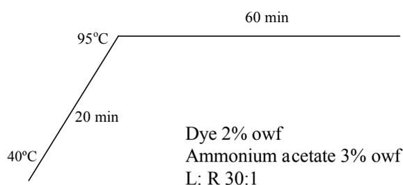
**Figure 3.** Dyeing method for Direct Green 6 on wool.
