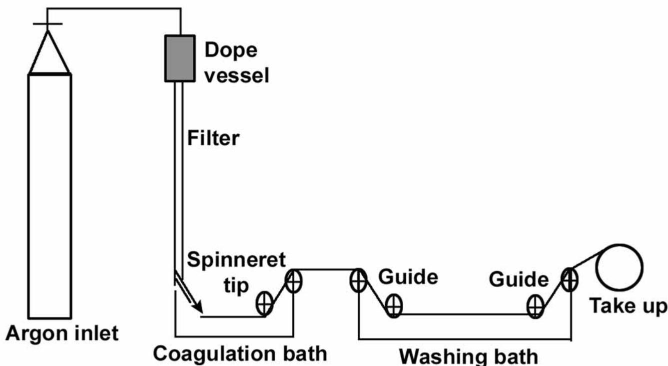
Figure 1. Schematic diagram for spinning fibres.
