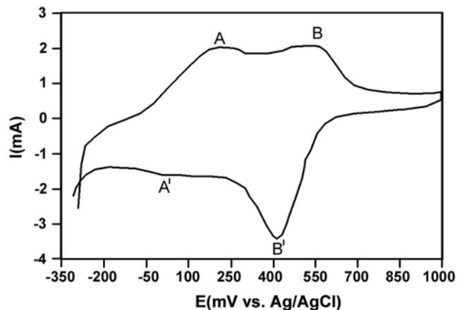
**Figure 4.** Cyclic voltammogram of fibre containing 25 % w/w of PANI. Scan rate 50 mV/s, electrolyte 0.1 M HCl.
