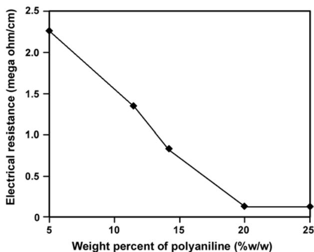
**Figure 3.** Variation of electrical resistance with increasing of PANI contents in blend. Data was plotted for fibres, which was placed 24 h at room temperature.
