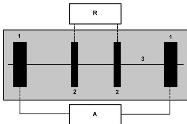
**Figure 2.** Schematic diagram for four-probe cell. (1) outer electrodes, (2) inner electrodes, (3) fibre sample, (A), galvanostat and (R) ohmmeter.
