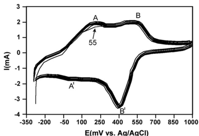
**Figure 5.** Cyclic voltammograms of fibres containing 25% w/w of PANI in various scans: 1, 5, 10, 15, 20, 30, 40, 50, 55. Scan rates 50 mV/s, electrolyte 0.1 M HCl.
