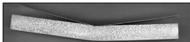
**Figure 5.** Failure mode of sandwich panel, sample 1.
