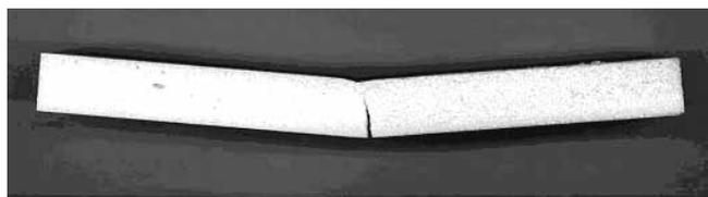
**Figure 4.** Failure mode of foam core alone.
