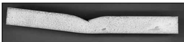
**Figure 8.** Failure mode of sandwich panel, sample 4.
