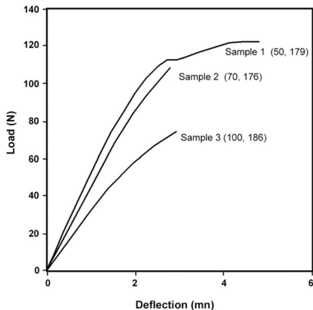
Figure 3. Load-deflection curves of core materials (the right hand side number in the parentheses is the foam core density ( $\text{Kg/m}^3$ ) and the left hand side number is the processing temperature in centigrade).
