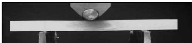
Figure 1. Sandwich beam loaded in flexural.
